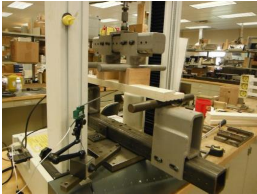
Photo No. 5 Flexural Properties Evaluation Test Setup
