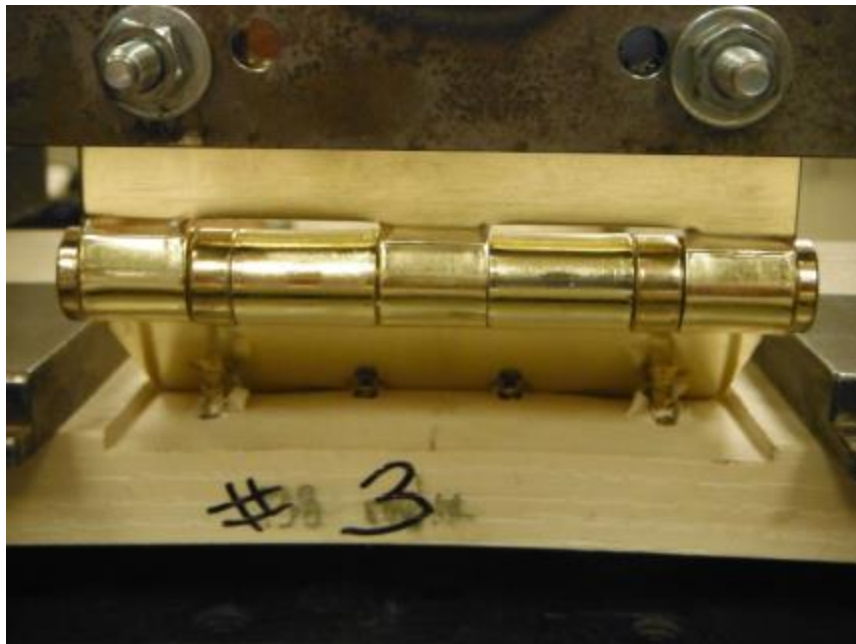
Photo No. 8 Hinge Loading Resistance Failure Detail (Typical)
