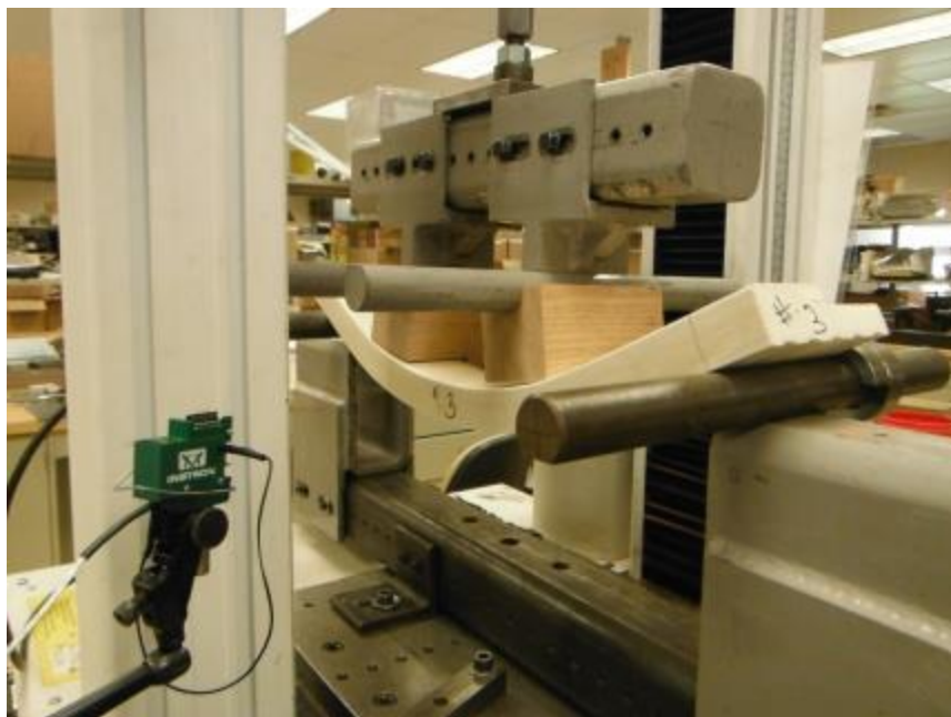
Photo No. 6 Flexural Properties Test Failure Detail (Typical)
